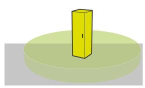
Area classification ZONE 2 inside the cabinet No area classification outside the cabinet the flashpoint is not sufficiently above the storage temperature (refer to TRGS 721, point 3.2 (3))
